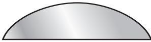
Eyebrow 4:1 Ratio Height must be less than 1/2 the base, but cannot be less than 1/4 of the base
